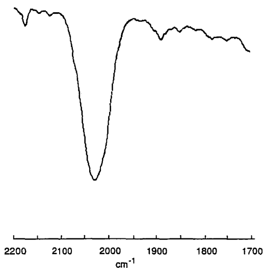
FIG. 2. Infrared absorbance of CO on isobutylaluminum-oxane-stabilized platinum colloid in methylcyclohexane solution.
